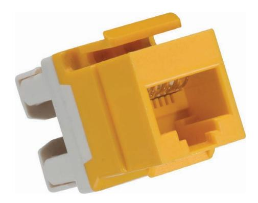
DIGILINK E400 unshielded copper RJ-45 keystone jack series includes high performance Category 5e+snap-in 8-position/8-contact (8P8C) jacks conforming to IEC 60603-7-2 (unshielded 100 MHZ connectors). DIGILINK E400 jacks are designed for fast and easy snap-in and out of wall plates and patch panels. All DIGILINK E400 jacks are designed in a 180° form and are available with back interconnection of 110 IDC blocks.
